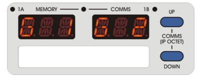
The red alphanumeric displays are now showing the three-character name for each audio channel. These are set from the master unit. If no names have been entered, the display will show "---"
